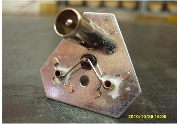
Open up a TV 2-way "splitter" (you can use any of two types as shown below) and remove the 75Ω resistors in series with each outlet. Wire all three solder points direct as shown. Make up a stub with any cable as described below.
